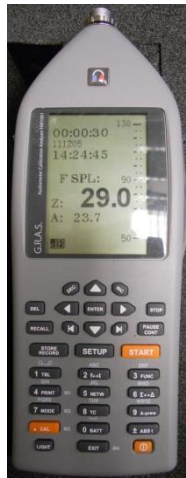
Sound Level Meter (G.R.A.S. HW1001)
