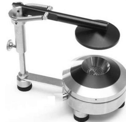
Test stand (G.R.A.S. RA0052) Artificial Ear (G.R.A.S. RA0039)
