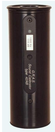
Microphone calibrator (G.R.A.S. 42AB)
