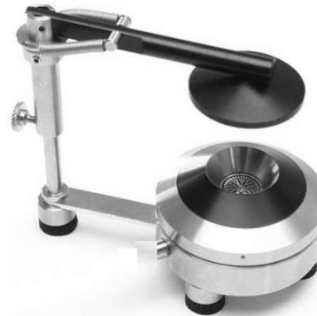
Test stand (G.R.A.S. RA0052) Artificial Ear (G.R.A.S. RA0039)
